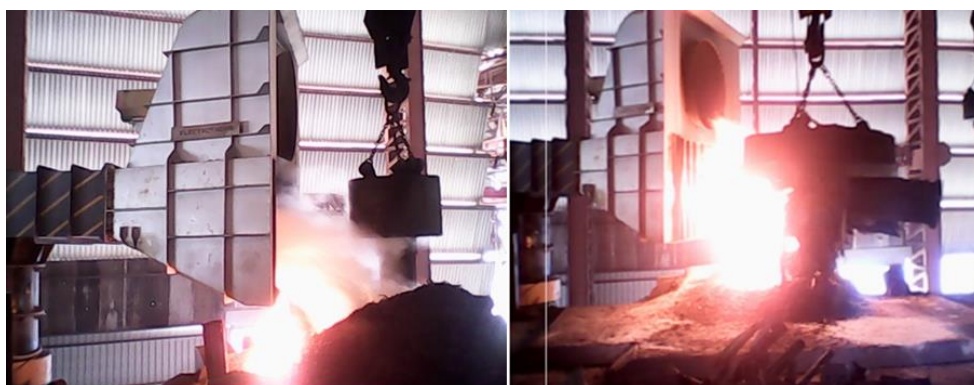
Figure 6.14: Working of side-based Suction Hood
